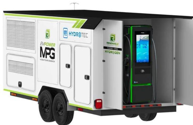
GM's Mobile Power Generator can fast-charge EVs without having to expand the grid or install permanent charge points in places where there is only a temporary need for power GM
