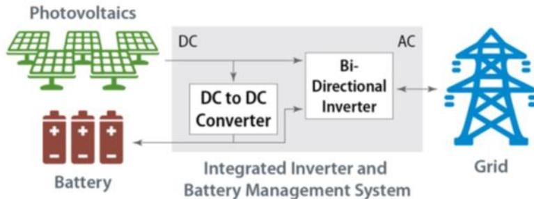
The DC coupling provides increased efficiency, and the grid charging provides more mission flexibility.
