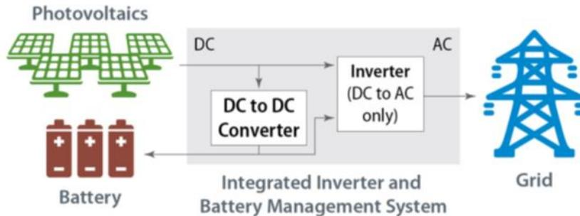
Both of the above configurations only have a single connection point to the grid. Depending on the size of the system, interconnection costs can make up anywhere from 20 to 35 percent of the balance-of-systems cost stack, and just having single point of interconnection reduces these costs (see chart in section 2.1).
